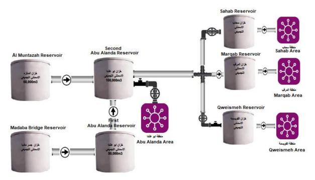
Figure 5-2: Schematic of Water Supply in Sahab - System One
