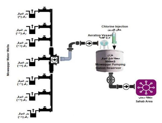
Figure 5-3: Schematic of Water Supply in Sahab – System Two
