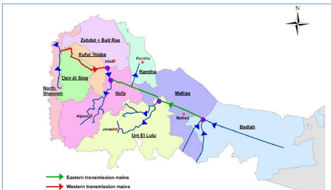
Figure 5-2: Water Transmission Mains in the Northern Regions
